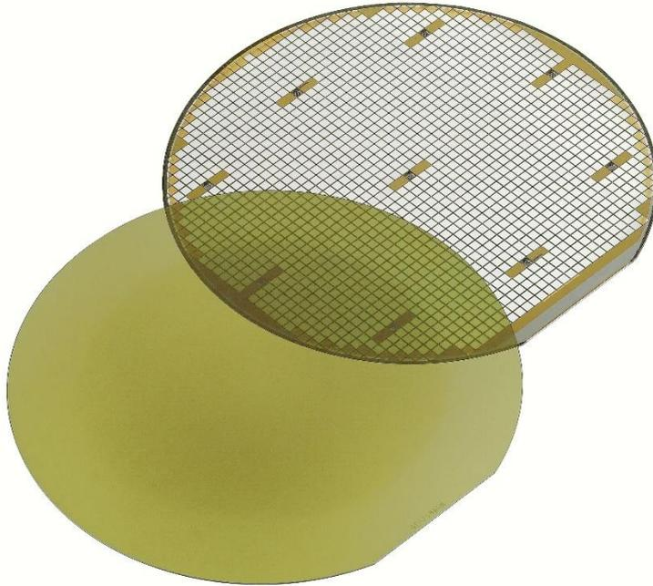
Fig1: SiC maturity on 6" wafers – comparison semitransparent SiC substrate vs completed product wafer
